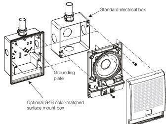
EDWARDS recommends that these speaker-strobes always be installed in accordance with the latest recognized edition of national and local codes. Refer to installation sheet for mounting height information.
